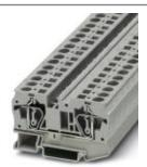
Feed-through terminal block, nom. voltage: 1000 V, nominal current: 41 A, connection method: Spring-cage connection, number of connections: 2, cross section: 0.2 mm² - 10 mm², AWG: 24 - 8, width: 8.2 mm, color: gray, mounting type: NS 35/7,5, NS 35/15
