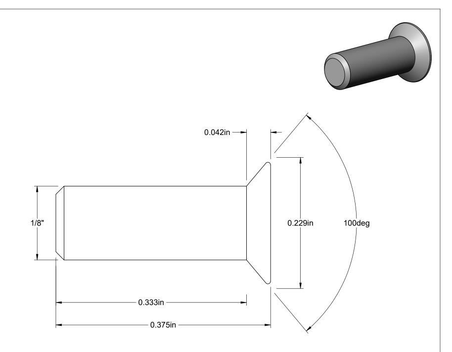
For Hole Size: 0.129in For Drill Bit Size: No.30
