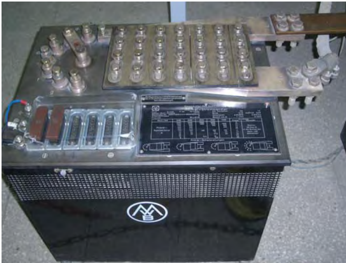
STANDARD TRANSFORMER RATIO ERROR \pm 0.005\% , PHASE ERROR \pm 0.5 MINUTES
